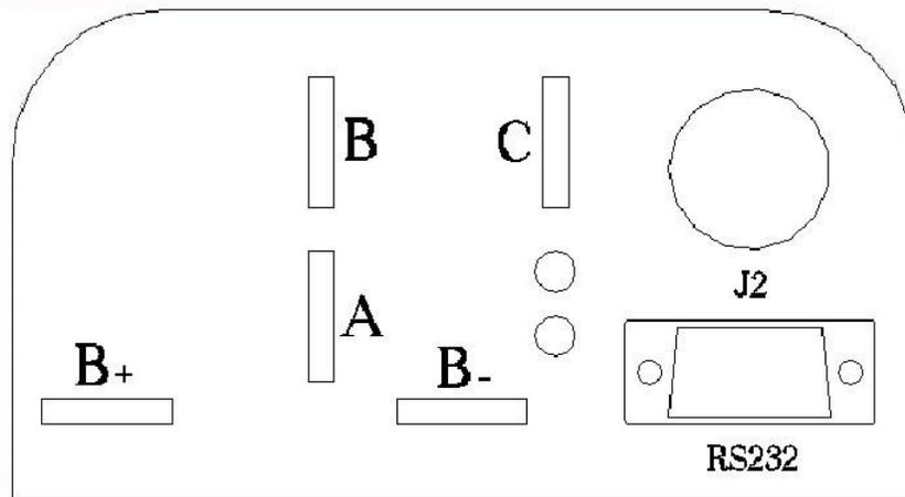
Figure 3: Brushless motor controller front panel
